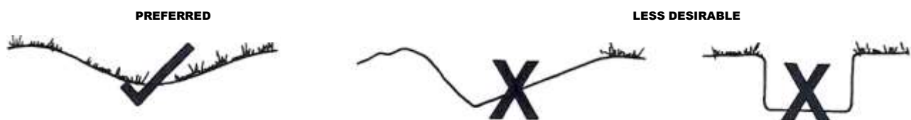
Figure 16. Grassed or Vegetated Swale Drain Formation
