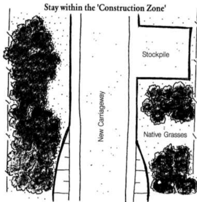
Figure 9. Clearly identify area of disturbance or machinery access or 'Construction Zone'.
