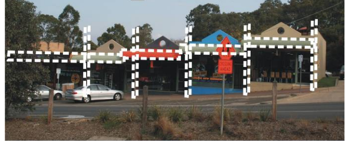
f wrap feature facade treatment to exposed side elevations
